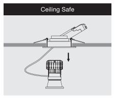
Reverse the installation step 4 for LED module replacement / maintenance.
