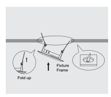
1. Cutout and fold up the spring clips and gently insert one side of the fixture into the cut out hole.
